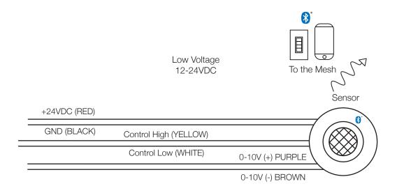
Control High Vin-2.5V 100mA Source Control Low - 100mA Sink
