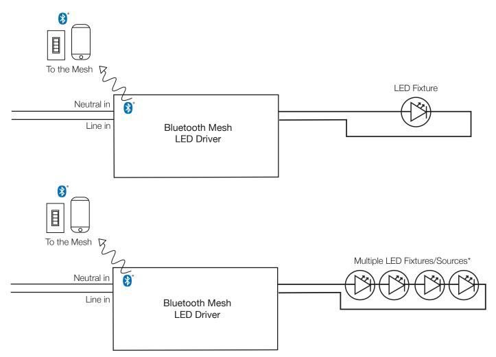
For best results, drivers need to be installed within 30 feet of the closest device within the Bluetooth Mesh network. Signal strength significantly decreases in presence of metal barriers such as when devices are enclosed in metal boxes.
