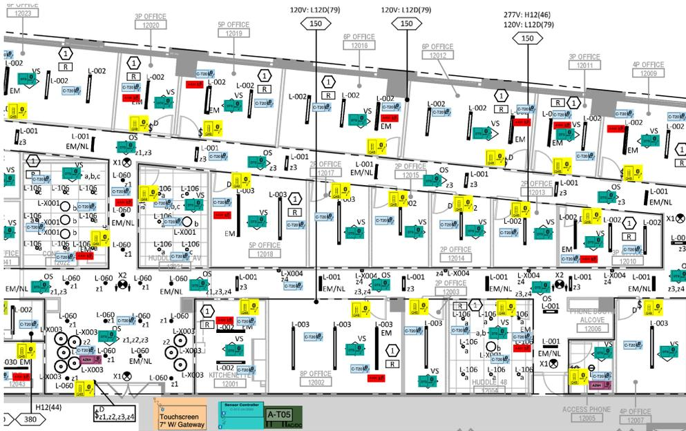
It is very important to install the devices on the establish location as this location will allow for the proper mesh network communication. A change in location could generate network malfunctioning.
