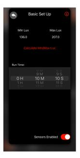
The following screen will require you to select a hold lux value and a value within the range. The slider would be set to the middle of the range by default.
