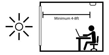
• Check that the daylight sensor's view is not obscured.
