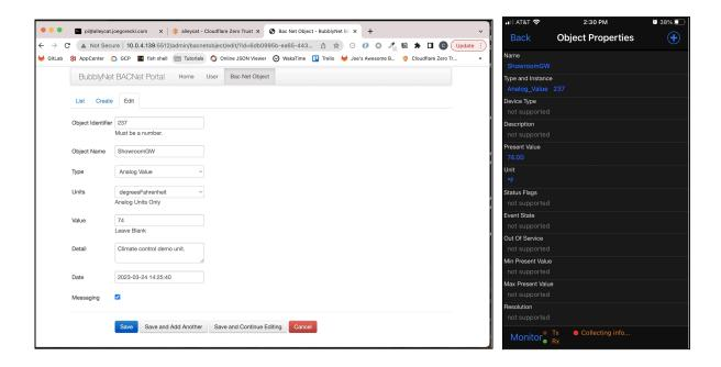
You can add a new object to the network by populating the provided webpage. The following fields are used to define the BACnet object:
