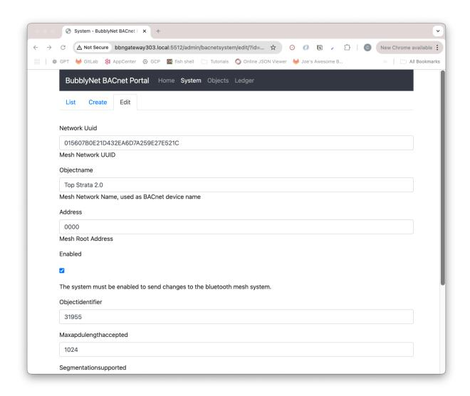
Warning: The entire system will be available with BACnet explorer but commands will not be relayed until the ENABLED is checked.
