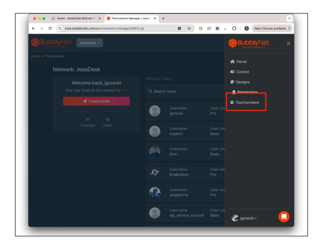
To configure the Bluetooth Mesh Gateway or Touchscreen Controller to work with the BACnet system, click the Touchscreens from the side or top navigation (depending on screen width).
