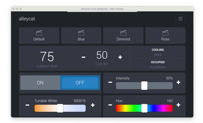
The Sample control panel in dark mode with CTL, HSL, Scene support, and HVAC controls. Click the control panel menu screen to change from Light Mode to Dark Mode or return to the Touchscreen setup system for system maintenance.
