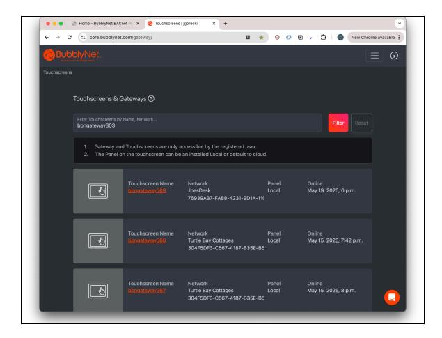
Find and choose the correct gateway that is going to to be configured for BACnet objects list. The touchscreen being used as a gateway is bbngateway303.
