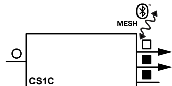
CS1C C-S1C-24-DS00 SENSOR/DRY-CONTACT CONTROLLER 3.25"x1.5"x0.25" (82.5x38x6.35mm) INPUT 12-24 VDC | OUTPUT 0-10VDC INSTALL WITHIN 60' OF CLOSEST DEVICE
